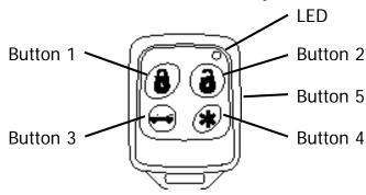
The ASTRA/G55 comes equipped with the 5-button Remote Transmitters used to control system operations.
