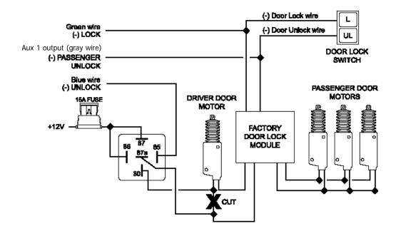
Two Stage Positive Trigger(using inverter)
